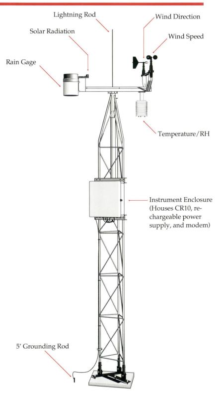
Tower height is 8'; an extendable 3' mast allows adjustment of sensor measurement heights. Optional solar panel is not shown.
