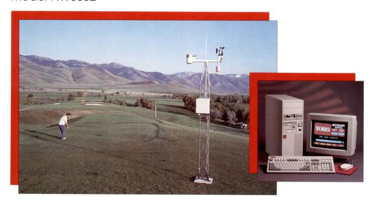
Turf grass water management is automated with Campbell Scientific's NW8002 Weather Station and Toro's Central Irrigation and Control Systems.\*
